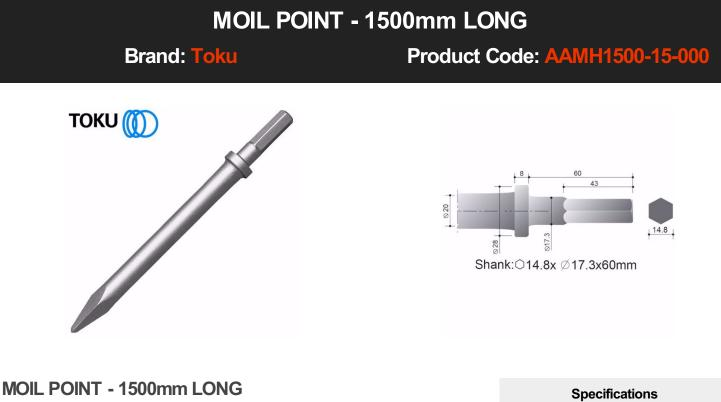
5/8" x 60mm Hex Shank Moil Point - 1500mm long chisel to suit a 5/8" hex industrial chipping hammer.
